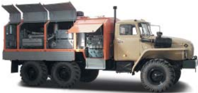
PKS-8/101 mounted on Ural truck chassis
