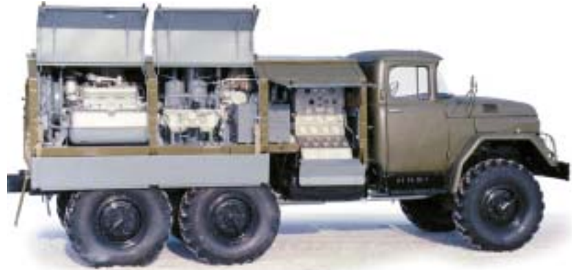
UKS-400V-131 mounted on ZIL-131 truck chassis
